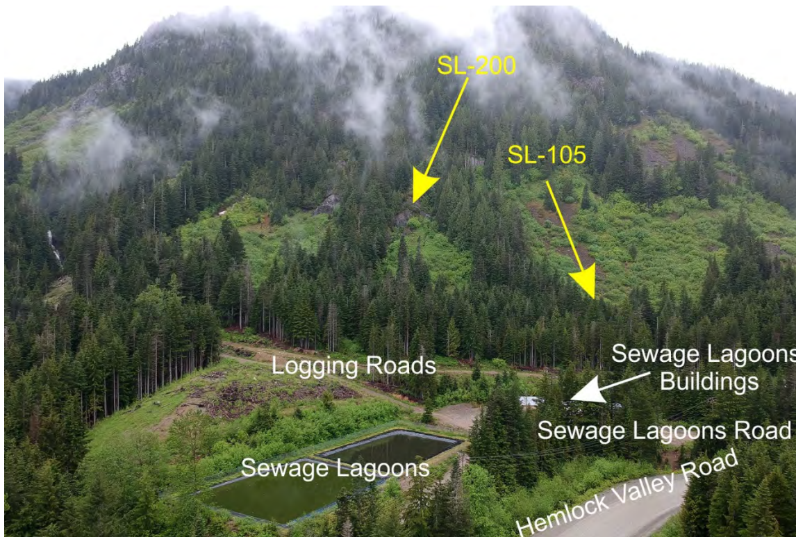
Photograph 12. Looking west towards paths SL-105 and SL-200 above the sewage lagoons and buildings. Avalanche paths exist adjacent to these paths but do not intersect the study area.
